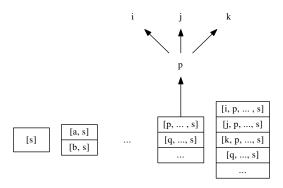
Figure 14.28: The stack is initialized with a singleton list of the starting point s. s is connected with point a and b. Paths  $\{a,s\}$  and  $\{b,s\}$  are pushed back. In some step, the path ended with point p is popped. p is connected with points i, j, and k. These 3 points are expanded as different options and pushed back to the stack. The candidate path ended with q won't be examined unless all the options above fail.
