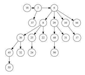
Figure 10.3: A binomial heap with 19 elements
