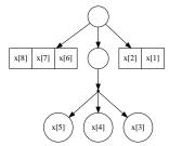
(c) Another element is remove from head. We borrowed one node from the middle part inner tree, change the node, which is a 2-3 tree to a list, and use it as the new front finger. the middle part inner tree becomes a leaf of one 2-3 tree node.
