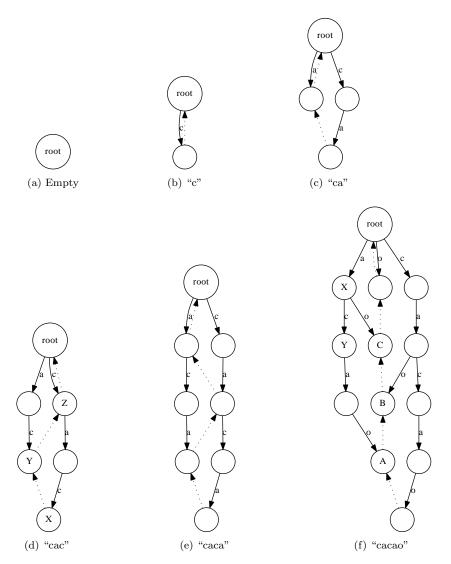
Figure 6.6: Construct suffix trie for "cacao". There are 6 steps. Only the last layer of suffix links are shown in dotted arrow.
