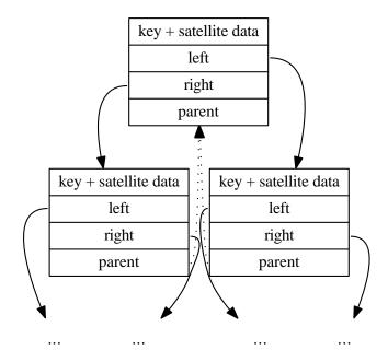
Figure 1.3: Layout of nodes with parent field.
