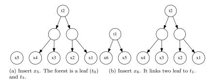
Figure 12.3: Steps of inserting elements to an empty list, 2
