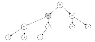
(a) Since 15 is greater than its parent 14, they are swapped. After that, because 15 is less than 16, the process terminates.
