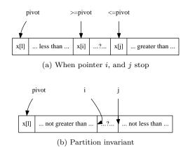
Figure 13.4: Partition a range of array by using the left most element as the pivot.
