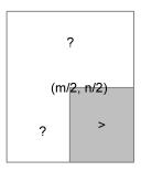
Figure 14.2: Left: the middle point element is smaller than x. All elements in the gray area are less than x; Right: the middle point element is greater than x. All elements in the gray area are greater than x.
