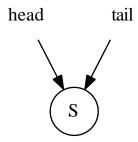
Figure 11.1: The empty queue, both head and tail point to sentinel node.
