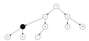
(c) Step 2, 16 is the largest element in current sub tree, next is to check node with value 2;
