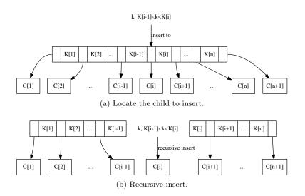
Figure 7.6: Insert a key to a branch node
