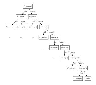
Figure 14.16: The infinite state tree for pattern 'ananym'.
