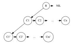
Figure 10.4: Example tree represented in 'left-child, right-sibling' way. R is the root node, it has no sibling, so it right side is pointed to NIL.  $C_1, C_2, ..., C_n$  are children of R.  $C_1$  is linked from the left side of R, other siblings of  $C_1$  are linked one next to each other on the right side of  $C_1$ .  $C'_2, ..., C'_m$  are children of  $C_1$ .
