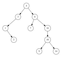
Figure 1.5: The successor of 8, is the minimum one in its right sub tree, 9; In order to find the successor of 2, we go up to its parent 1, but 1 doesn't have left child, we go up again and find 3. Because its left child is also the ancestor of 2, 3 is the result.
