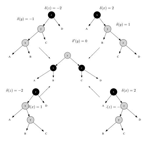
Figure 4.3: 4 cases for balancing a AVL tree after insertion
