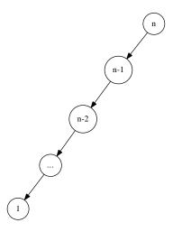
(b) The partition tree for  $\{y_1 > y_2 > ... > y_n\}$ , There aren't any elements greater than or equal to the pivot (the first element) in every partition.
