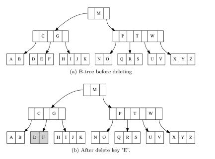
Figure 7.19: Result of delete-then-fixing (1)
