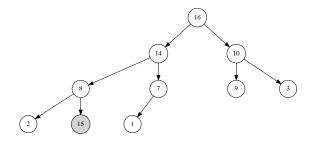
(b) The key is modified to 15, which is greater than its parent;
