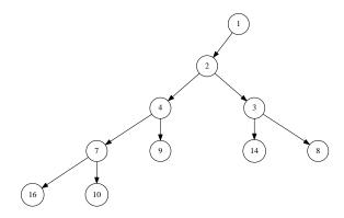
Figure 8.12: Skew tree is still balanced even the input is an ordered list  $\{1, 2, ..., 10\}$ .
