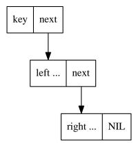
Figure 1.4: Binary search tree node layout on top of linked list. Where 'left...' and 'right ...' are either empty or BST nodes composed in the same way.
